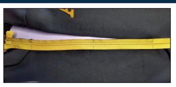
Close the zipper and mark the places for the hood attaching seam, waist mark and zipper bottom mark on the other zipper tape.
