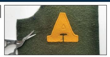
Working on the wrong side, trim the excess fabric close to the stitching.
