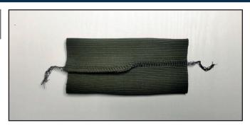
To avoid excess thickening when stitching the cuffs, press the seam allowances in different directions.
