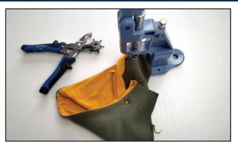
Punch 3 mm (1/8") holes for the grommets with a Hole Punch or scissors. Attach the grommets with a press.
