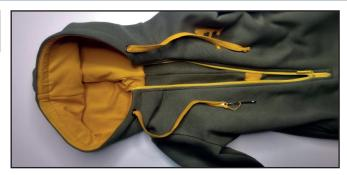
Insert the flat cord, tie the seam thread tails, trim the excess cord close to the knots.
